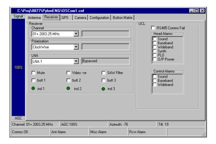
This form provides indication of the current receiver features selected, together with the condition of three spare relay controls. The check box indicators are ticked if a control output is currently active and the operator can click on these controls to operate the mute, video invert, saw filter, spare 1, spare 2 and spare 3 control outputs, which all operate as latching push-buttons.
