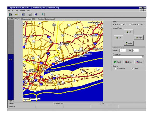
This form allows the user to control both steerable and horn antennae using user-configurable BitMaps for convenience. In normal operation the user drags the azimuth pointer on the display to the correct area of transmission and then releases to signal the outstation to automatically steer to that point.
