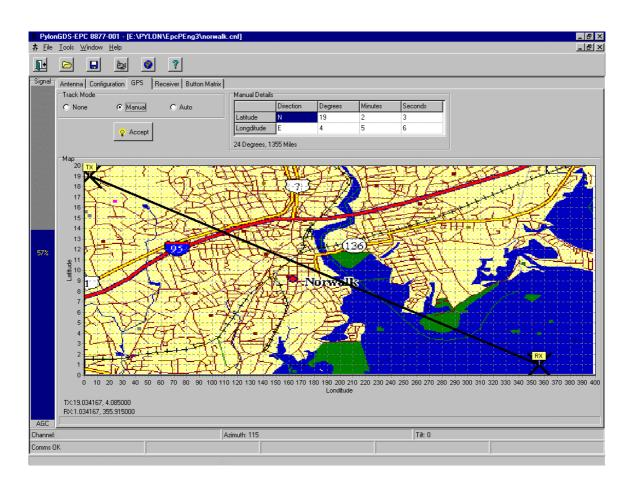
This form allows the user to make full use of GPS information. In Manual mode of operation, if the transmit site Lat./Long is given to the user he can simply enter this into the control system to
