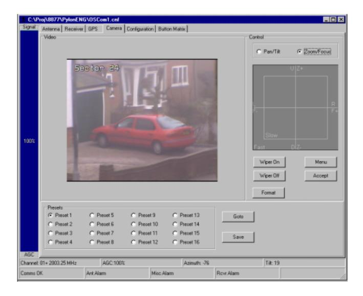
If a camera option has been configured, this form allows the user to control the camera mount and in addition (if a video for windows compatible capture card is fitted) will allow the video to be previewed.
