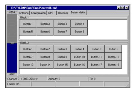
PylonGDS-ENG3 allows the control of other system functions using powerful user-configurable push-button grids. The buttons have configurable legends, colors, bitmaps and multi-action
